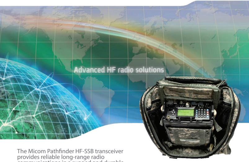
The Micom Pathfinder HF-SSB transceiver provides reliable long-range radio communications in a rugged and durable backpack configuration built to withstand severe shock, vibration, and extreme weather conditions. The lightweight Homeland Security version of the Micom, the Pathfinder, makes it especially suitable for users who carry out on-foot field operations.
