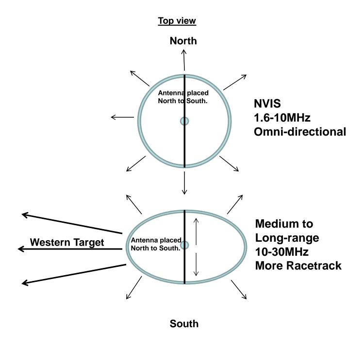
Power concentrated to east and west (10-30 MHz) with antenna setup running North to South. Antenna is placed north to south to take advantage of the Racetrack pattern/power to the east and west. Antenna is placed running East to west for racetrack pattern/power to North and South.
