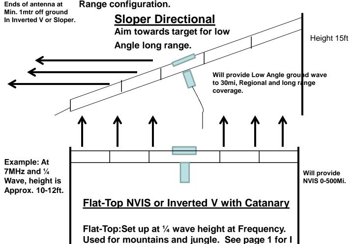
Inverted V with catenary set up.
