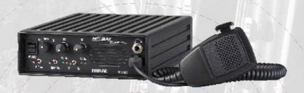
The MICOM-LINK is a cross band repeater unit that provides manually determined interconnectivity between HF/SSB and UHF/VHF radios. It is most commonly used to provide a communications path from local area UHF/VHF FM handie-talkies through the AM HF/SSB long-haul backbone to a Communications Center offen hundreds of miles distant.
